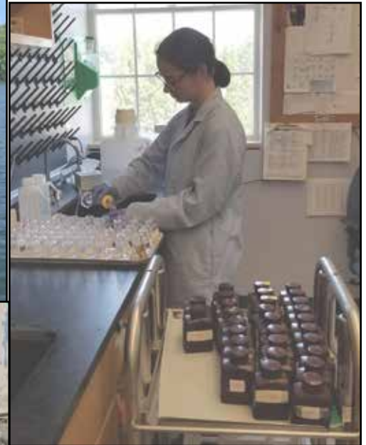
Above; Tehya Kloster measures water samples for the phosphorous test and pours them into flasks to be autoclaved.
